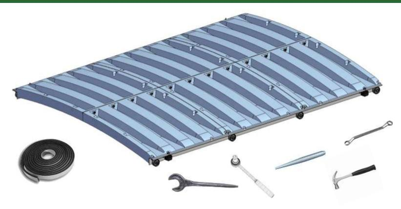
To assemble the STD lid sections you will need:- 19mm socket and wrench, a "rats-tail" spanner or taper drift, hammer and a 19mm ring spanner. Ensure a roll of seal strip is available as per kit list. The ideal place to assemble is at the side of a dock loader or a safe raised platform of some kind around 1200mm high. It is necessary to have two men do this task as the sections need to be held steady during assembly and care must be taken at all times.
