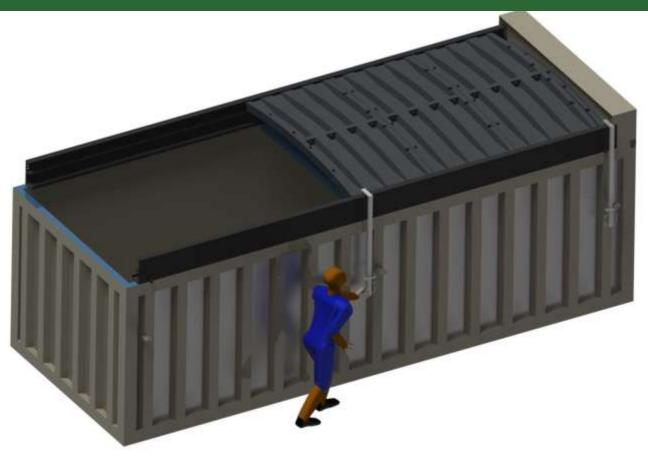
The lids should traverse back and forth without snagging, and if so channel frame end section can be fitted. If lids do not travel smoothly you have got something wrong and need to check all dimensions of channels etc. and wheel and handle fittings.
