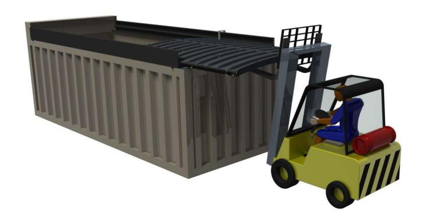
One man drives the fork-truck and a second man pushes the handle to ensure the **bottom** lid section is entered properly into the channel frames. The handle should be at the furthermost point from the fork truck.
