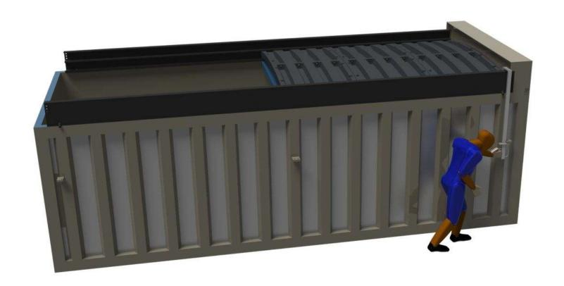
Once this lid section is fully home and secure, the top section can be fitted.
