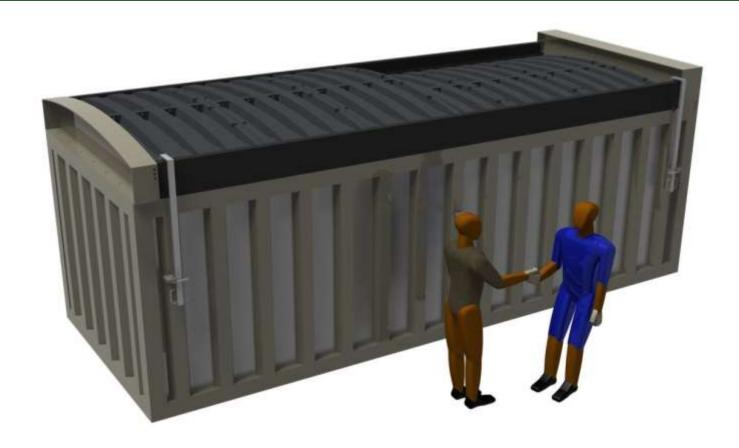
Final check on lid travel and if OK a job well done! Please ensure during use no deposits of any kind build up in the channels, the water drainage is working and no material is tipped on the closed lids by mistake.
