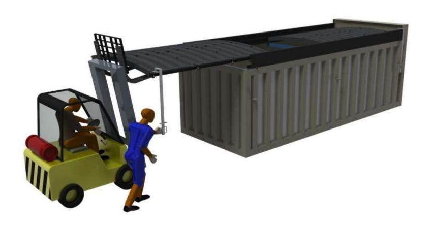
This top section is positioned same as first but with handle at the innermost point from the fork truck, this can be used to steady the lid section as its entered.
